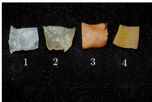
Figure 15. Physical aspect of the final product of aluminum selective membrane. (1) StyrenegraftedPP-1, with high yield of grafting (not chemically modified). (2) Chemically modified PP-1 (low yield - first step of modification). (3) Chemically modified PP-1 (high yields - first step of modification and grafting). (4) Chemically modified PP-2 (high yield for the first modification and low yield of grafting).
