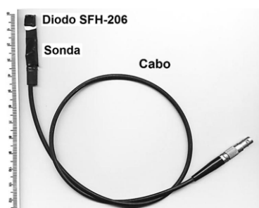
Figure 3. Low-cost pin diode dosimeter probe.
