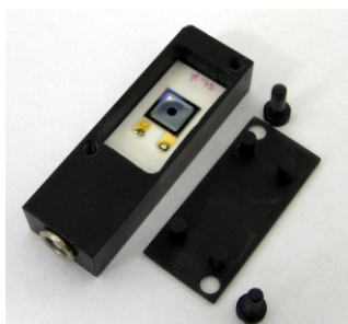
Figure 4. Epitaxial radiation-hard Si diode probe.
